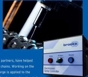
develop Electrostatic Lubrication for pin oven chains. Working on the principle of 'opposites attract', a negative charge is applied to the lubricant as it flows from the nozzle causing the stream to be attracted to the chain like a magnet. Once the lubricant hits the chain the negatively charged oil particles disperse into the chain direct to the bearing surfaces.
